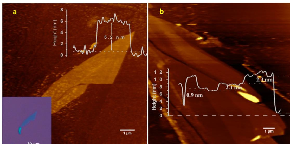
**Figure 2.** AFM image of exfoliated InSe flakes. (a) Flake with a thickness of 5.2 nm, which corresponds to four to five layers. (b) Thinner flake with varying thickness. The thickness of the flake varies from 6 to 12 nm, with a step height of 2 nm, which corresponds to two layers.
